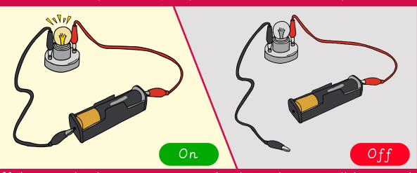
If there is a break in a series circuit, the electrical current will be cut and all the components will stop working. Causing a break in a series circuit can act as a switch to turn the circuit off.
